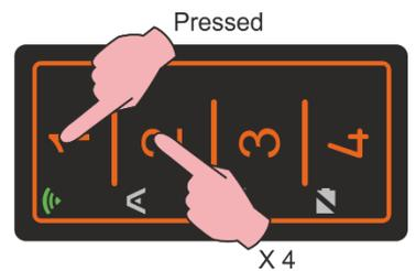
**Step 2:** release the keys and place the HÖRMANN remote control in front of the FACILE PRO at a distance of about (2÷4) cm.
