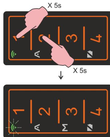
**Step 2:** press and hold down the key of the FACILE PRO whose source code you want to send. The **TX** LED stays on for about six seconds, equivalent to the time the source code is sent.
