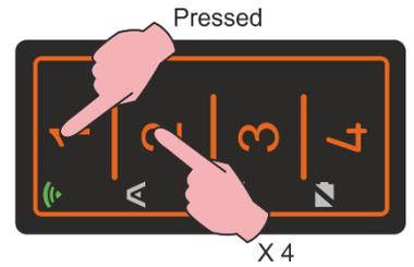
**Step 4:** release the keys and place the CAME remote control in front of the FACILE PRO at a distance of about (1÷4) cm.
