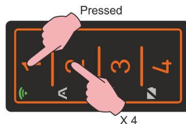
**Step 2:** release the keys and place the fixed code remote control in front of the FACILE PRO at a distance of about (1÷4) cm.
