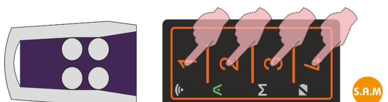
**Step 6:** the copy is completed, the FACILE PRO key containing the V2 code needs to be memorized in the original receiver with the S.A.M. procedure (\*).
