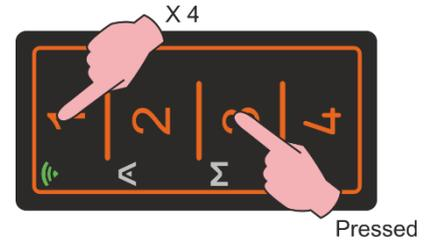
**Step 2:** release the keys and place the original remote control in front of the FACILE PRO at a distance of about (1÷4) cm.
