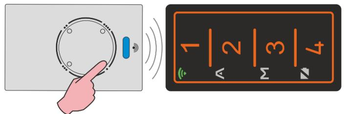
**Step 4:** the TX LED starts to flash twice. Move the two remote controls away, press and hold down keys 1 and 2 of the F/G remote control simultaneously for about three seconds, then release them. The remote control LED starts flashing.
