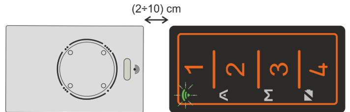
**Step 3:** press and hold down the key of the F/G remote control until the FACILE PRO TX LED stays on steadily, then release it.
