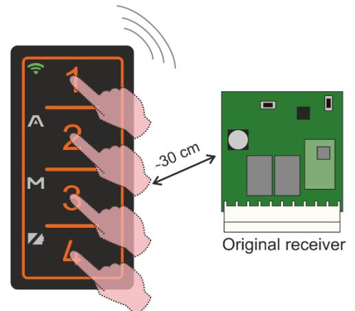
**Step 3:** manual memorization is completed. Press the key just memorized several times to check correct operation between FACILE PRO and the original receiver.
