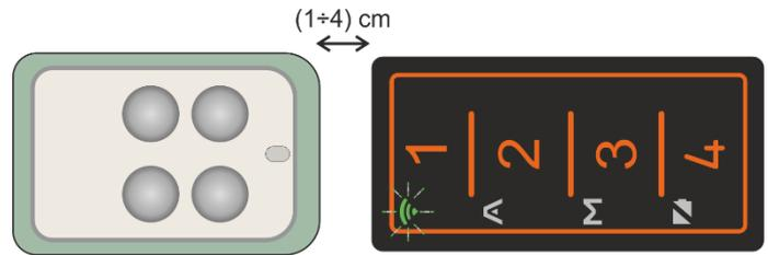
**Step 3:** press and hold down the key of the original remote control until the FACILE PRO TX LED starts flashing quickly, then release it.
