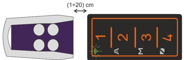
**Step 3:** press and hold down the key of the V2 remote control until the FACILE PRO TX LED stays on steadily, then release it.
