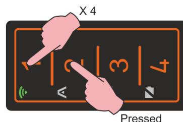
**Step 2:** release the keys and place the original remote control in front of the FACILE PRO at a distance of about (1÷4) cm.
