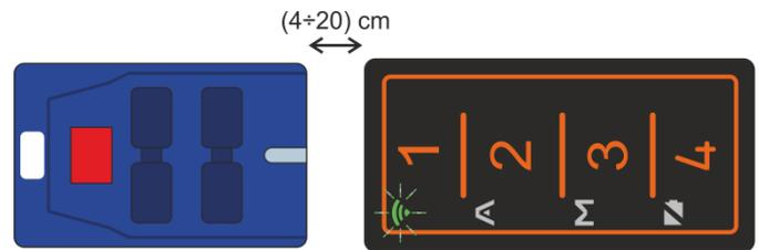
**Step 3:** press and hold down the key of the BFT remote control until the FACILE PRO TX LED stays on steadily, then release it.
