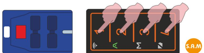
**Step 6:** the copy is complete, the FACILE PRO key containing the BFT code needs to be memorized in the original receiver with the S.A.M. procedure (\*). Consult the paragraph "S.A.M. SELF-MEMORIZATION" to memorize the FACILE PRO key in the original receiver.
