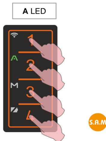
The copy is complete, the FACILE PRO key containing the code of the remote control just copied needs to be memorized in the original receiver with the S.A.M. procedure (\*). Consult "S.A.M. SELF-MEMORIZATION" paragraph to memorize the key of the FACILE PRO in the original receiver.
