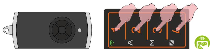
**Step 6:** the copy is completed, the FACILE PRO key containing the HÖRMANN code is immediately working with the original receiver (\*).
