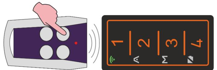
**Step 4:** the TX LED starts to flash twice. Press and hold down the same key of the V2 remote control pressed previously until the FACILE PRO TX LED starts flashing quickly, then release it.
