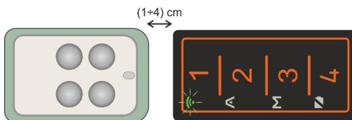
**Step 3:** press and hold down the key of the original remote control until the FACILE PRO TX LED starts flashing quickly, then release it.
