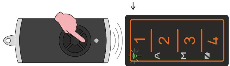
**Step 4:** the LED of the HÖRMANN remote control starts to flash blue and red alternately. Continue to hold the key until the FACILE PRO TX LED starts flashing quickly, then release it.
