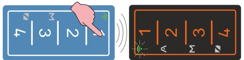
**Step 4:** now press the key of the FACILE PRO for memorize all keys of original remote control and check which LED lights up for a few seconds:
