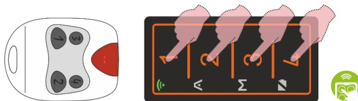
**Step 5:** the copy is completed, the FACILE PRO key containing the code of the remote control just copied is immediately working with the original receiver (\*).
