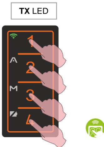
The copy is complete, the FACILE PRO key containing the code of the remote control just copied is immediately functional with the original receiver (\*). Press the FACILE PRO key several times to check correct operation between the remote control and the original receiver.
