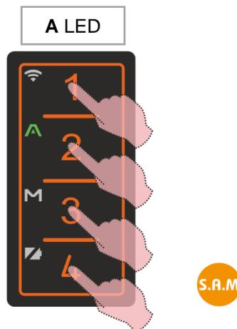
The copy is completed, the four keys of the FACILE PRO containing the code of the remote control just copied needs to be memorized in the original receiver with the S.A.M. procedure (\*). Consult "S.A.M. SELF-MEMORIZATION" paragraph to memorize the keys of the FACILE PRO in the original receiver.
