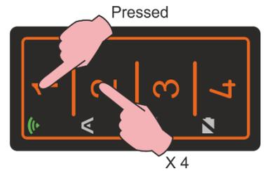
**Step 2:** release the keys and place the BFT remote control in front of the FACILE PRO at a distance of about (4±20) cm.
