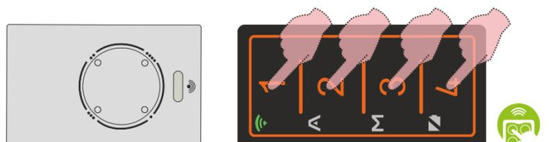
**Step 7:** the copy is completed, the FACILE PRO key containing the F/G code is immediately working with the original receiver (\*).
