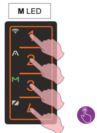
The copy is completed, the four keys of the FACILE PRO containing the code of the remote control just copied needs to be memorized manually in the original receiver. Consult "RECEIVER PROGRAMMING" paragraph to memorize the keys of the FACILE PRO in the original receiver.
