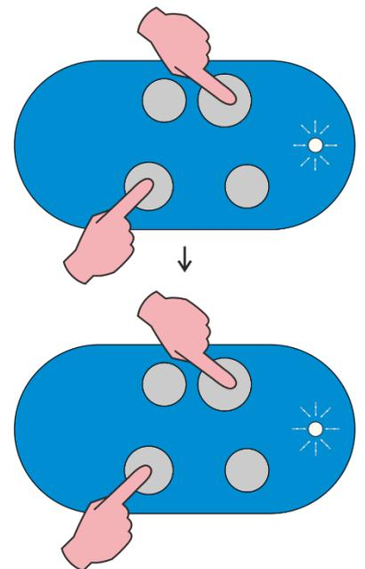
**Step 2:** once the quickly flashing has finished, the white LED of the CAME signals the currently set mode based on its behavior:
