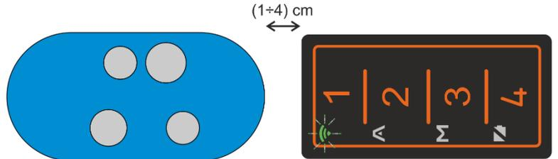
**Step 5:** press and hold down the key of the CAME remote control until the FACILE PRO TX LED starts flashing quickly, then release it.
