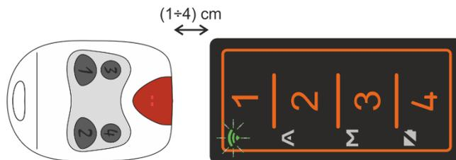
**Step 3:** press and hold down the key of the fixed code remote control until the FACILE PRO TX LED starts flashing quickly, then release it.
