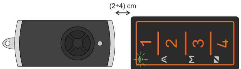
**Step 3:** press and hold the key of the HÖRMANN remote control. The blue LED lights up for about 3 seconds, then turns off.
