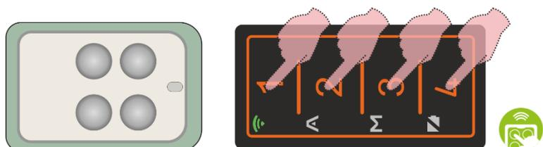
**Step 5:** the copy is completed, the FACILE PRO key has the same serial code (Rolling-code) as the remote control just copied and is therefore immediately functional with the original receiver (\*).
