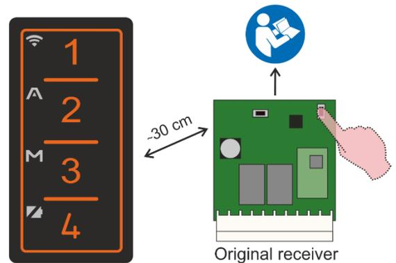
**Step 2:** press and hold down the key of the FACILE PRO that you want to memorize until the original receiver decodes the code, then release it.
