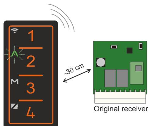
**Step 3:** self-memorization is completed. Press the key just memorized several times to check correct operation between FACILE PRO and the original receiver.
