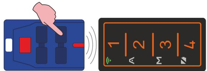
**Step 4:** the TX LED starts to flash twice, now send the source code of the BFT remote control by pressing the key hidden on the back or, in the case of more recent models, by keeping keys 1 and 2 pressed simultaneously until the FACILE PRO TX LED start flashing quickly, then release them.
