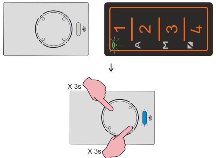
**Step 5:** reposition the F/G remote control in front of the FACILE PRO and send the source code by holding down the key to be copied until the FACILE PRO TX LED starts flashing quickly, then release it.
