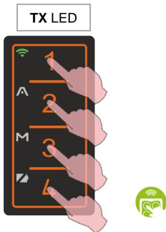
The copy is completed, the four keys of the FACILE PRO containing the code of the remote control just copied are immediately functional with the original receiver (\*). Press the FACILE PRO keys several times to check correct operation between the remote control and the original receiver.
