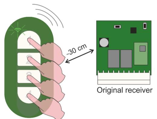
**Step 3:** manual memorization is completed. Press the key just memorized several times to check correct operation between AVATAR and the original receiver.
