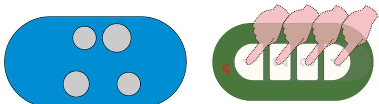
**Step 7:** the copy is completed, the AVATAR's key containing the CAME code needs to be memorized in the original receiver with the S.A.M. procedure (\*).
