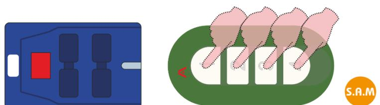
**Step 6:** the copy is complete, the AVATAR's key containing the BFT code needs to be memorized in the original receiver with the S.A.M. procedure (\*).
