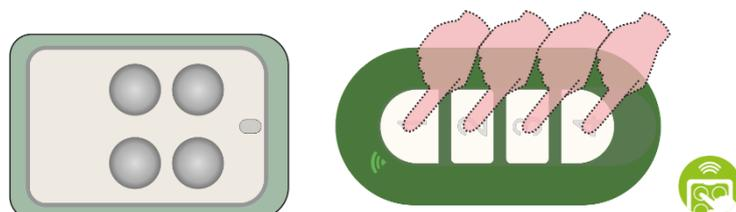
**Step5:** the copy is completed, the AVATAR's key has the same serial code (Rolling-code) as the remote control just copied and is therefore immediately functional with the original receiver (\*).
