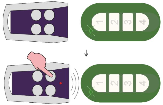
**Step 4:** the **TX** LED starts to flash twice. Press and hold down the same V2 remote control's key pressed previously until the AVATAR's **TX** LED starts flashing quickly, then release it.
