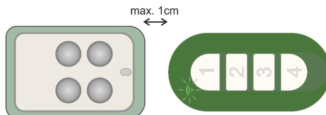
**Step 3:** press and hold down the original remote control's key until the AVATAR TX LED starts flashing quickly, then release it.
