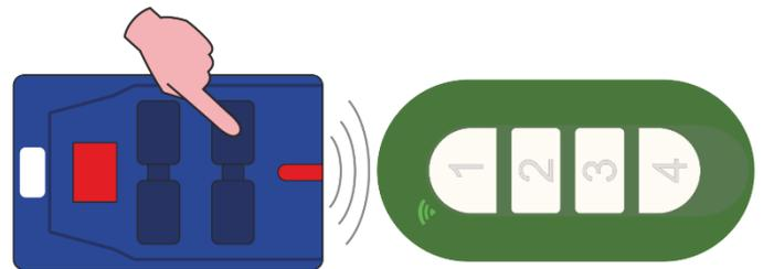
**Step 4:** the TX LED starts to flash twice, now send the BFT remote control's source code by pressing the key hidden on the back or, in the case of more recent models, by keeping keys 1 and 2 pressed simultaneously until the AVATAR's TX LED starts flashing quickly, then release them.
