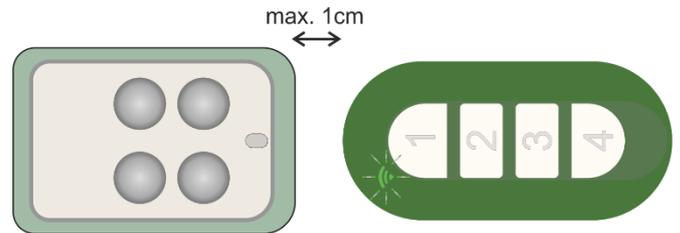
**Step 3:** press and hold down the original remote control's key until the AVATAR's **TX** LED starts flashing quickly, then release it.
