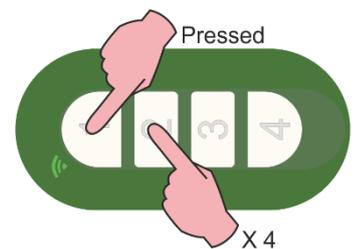
**Step 2:** release the keys and place the F/G remote control in front of the AVATAR at a distance of about 1cm.
