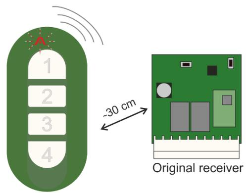
**Step 3:** self-memorization is completed. Press the key just memorized several times to check correct operation between AVATAR and the original receiver.
