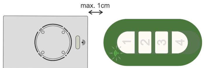
**Step 3:** press and hold down the F/G remote control's key until the AVATAR's TX LED stays on steadily, then release it.
