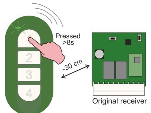
**Step 2:** after 8 seconds the **A** LED starts flashing quickly, release the key and wait for the LED to switch off.
