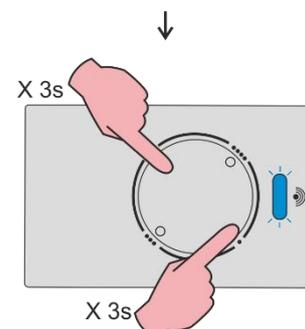
**Step 5:** reposition the F/G remote control in front of the AVATAR and send the source code by holding down the key to be copied until the AVATAR's **TX** LED starts flashing quickly, then release it.
