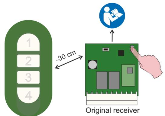
**Step 2:** press and hold down the AVATAR's key that you want to memorize until the original receiver decodes the code, then release it.
