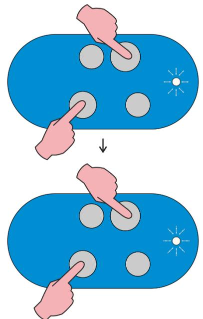
**Step 1:** press and hold down **1** and **2** CAME remote controls' keys simultaneously. The white LED starts to flash slowly, after about 4 seconds it starts to flash quickly.
