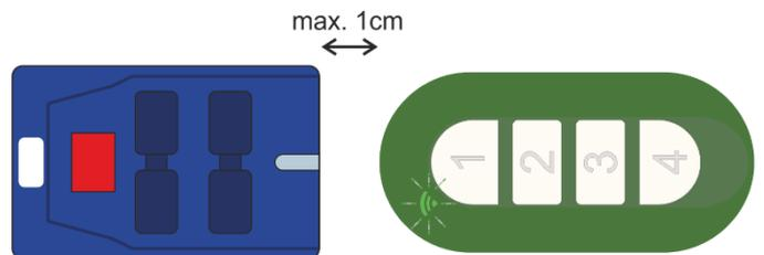
**Step 3:** press and hold down the BFT remote control's key until the AVATAR TX LED stays on steadily, then release it.
