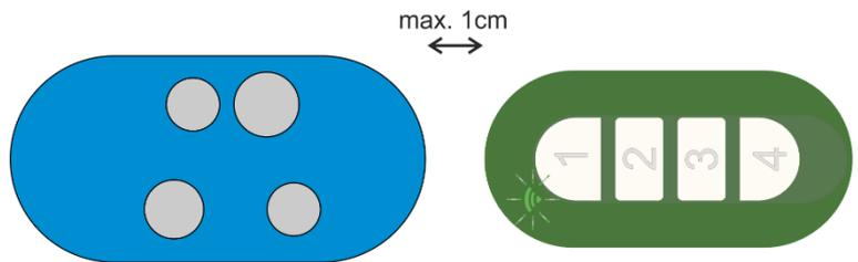
**Step 5:** press and hold down the CAME remote control's key until the AVATAR TX LED starts flashing quickly, then release it.
