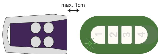
**Step 3:** press and hold down the V2 remote control's key until the AVATAR's **TX** LED stays on steadily, then release it.
