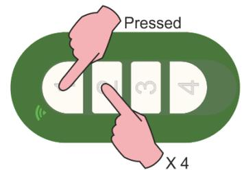
**Step 4:** release the keys and place the CAME remote control in front of the AVATAR at a distance of about 1cm.
