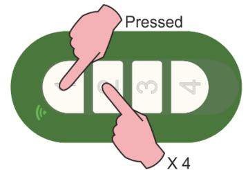
**Step 2:** release the keys and place the BFT remote control in front of the AVATAR at a distance of about 1cm.
